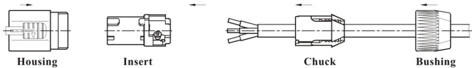
Put bushing and chuck onto the cable.
