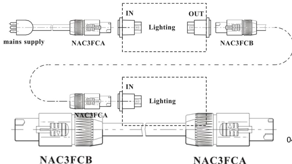
The power cable must be a three-conductor 2.5mm<sup>2</sup> cable.
