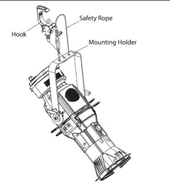
Please use qualified safety-rope, which can hold at least 10times the weight of the fixture. You must only use only safety-ropes with quick links with screw cap.
