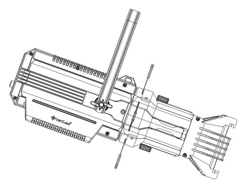
When rigging the devices on the truss and the head face to the floor. Insert the quick-lock fasteners of the first mounting holder into the respective holes on the bottom of the device. Tighten the quick-lock fasteners fully clockwise. Install the second mounting holder. And the safety rope must be used at same time.
