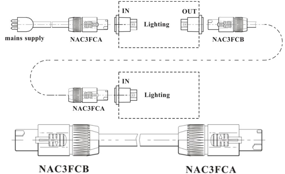
The power cable must be a three-conductor 2.5mm<sup>2</sup> cable.
