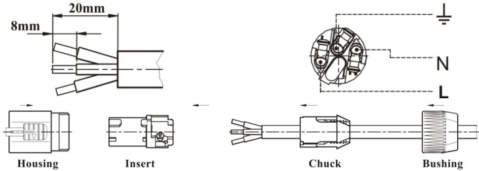
Put bushing and chuck onto the cable.
